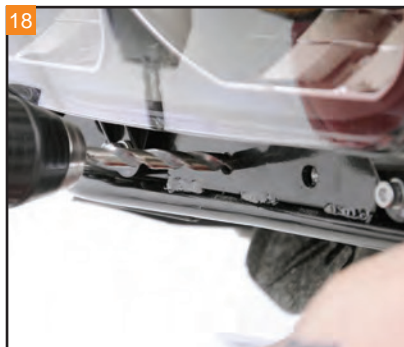
18 Enlarge the holes until they are large enough for a 5/16" bolt.
