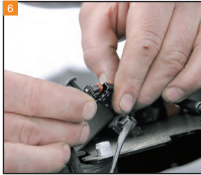
Unplug the connectors for the front turn signals.
