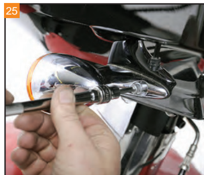
25 With a 3/16" Allen wrench, install the bolts behind the front turn signals.
