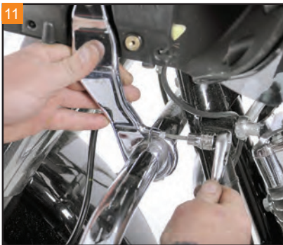
Remove the support brackets from the engine guard with a 5/32" Allen wrench.
